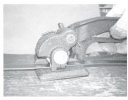
Compress the Handle (#1) to lift Support Frame (#8). While in this position, move the tool and slide the strap into the gap below the Feedwheel (#12). The strapping material is now locked and ready to be tightened.
