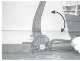
Hold the tool with your left hand and pump the Handle (#1) until the straps are sufficiently tight. Don't overtighten the straps as damage may occur to the tool and object being strapped.
