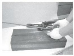
Place the strap around the object you wish to secure as shown. The end of strap is underneath.
