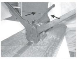
Open the sealer (not included) fully open position, put the sealer on the top of the seal, press the sealer handle together to fully crimp the seal, then remove the sealer.
