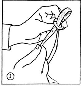
Insert loop through center of buckle. Bend BOTTOM line into loop. Pull down on strap coming from coil to tighten buckle.
