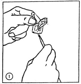
Make 3" fold-over with strap end. Insert folded end UP through center of buckle. Bend TOP line into folded strap end. Pull on folded strap to secure line.
