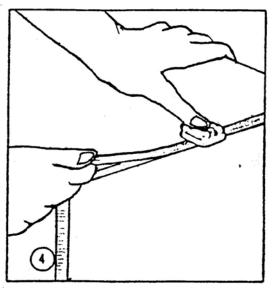
Apply pressure to top of the buckle with thumb to engage spacer between lines. Tighten strap.
